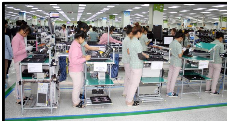
Mobile phone assembly at Samsung Electronics in Vietnam happens standing up. Photo credit: http://www.koreaherald.com/view.php?ud=20141111000954
