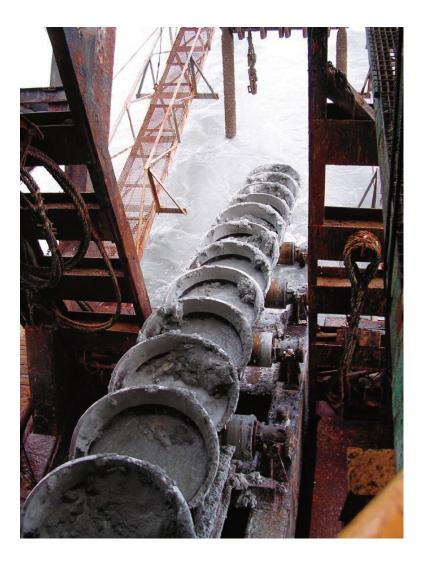
PT Timah's bucket ladder dredger dredging tin sand from the seabed.
