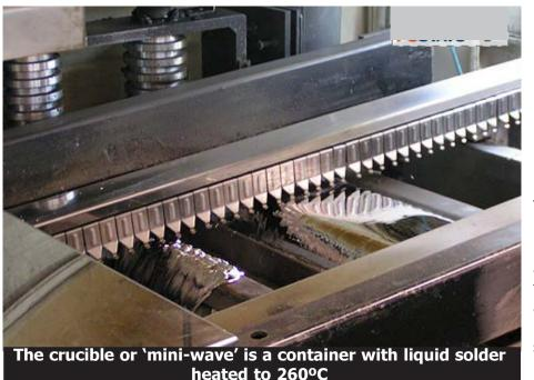
very bad. After taking the card out of the crucible, we do some final touches, again with solder and flux, and clean it up with isopropilic alcohol."
