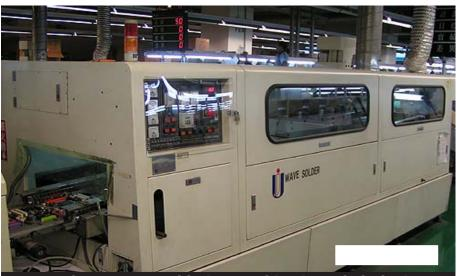
Even when a wave soldering machine is sealed, the input and output conducts are open. And there is where the fumes escape.
