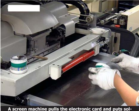
A screen machine pulls the electronic card and puts soldering paste on it. In the case of Ramona, the machine also caught her hand
